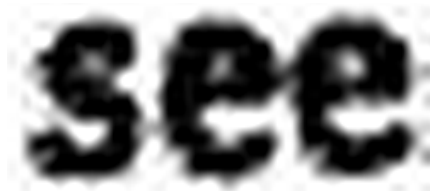
Figure 2b Actual image from a small, $50, 18MP image sensor with small, 1.25um x 1.25um pixels
